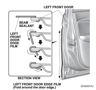
8. Using a shop towel, wipe the excess 3M protective tape application solution from the left front door edge film. Allow the left front door edge film to dry thoroughly.
