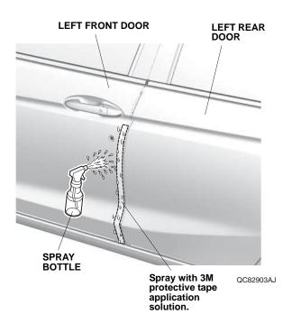
3. Open the left front door. Peel back about 50 mm (2.0 in.) of adhesive backing from the left front door edge film. Align the V-notch with the bottom of the character line on the left front door as shown.
