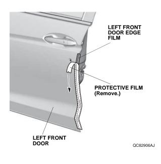
7. Starting from the center and working outward, use your fingers to fold the left front door edge film around the edge of the left front door as shown. Move your fingers in one direction only. Attach the left front door edge film over the seam sealant. Do not trim or damage the seam sealant.
