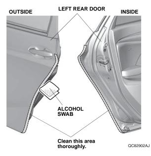
2. Close the left front door and left rear door. Using a spray bottle with 3M protective tape application solution, spray the area where the left front door edge film will attach.
