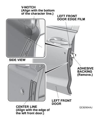
4. Align the center line on the left front door edge film with the edge of the left front door. While applying light pressure, carefully remove the adhesive backing, and attach the left front door edge film to the left front door. 5. Insert the applicator into the soft sleeve. Starting from the top and working downward, use the soft sleeve to smooth the left front door edge film. Move the soft sleeve in one direction only.
